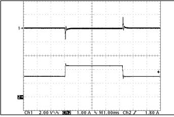
Figure 5: Output response to load current step for QTC version of product (50 %- 75 % -50 % of lout(max);  $dI/dt = 0.1 A/\mu s$ ). Load cap: 15  $\mu$ F tantalum cap and 1  $\mu$ F ceramic cap. Ch 1: Vout (2 V/div), Ch 2: lout (1 A/div).
