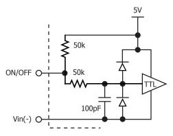
Figure B: Internal ON/OFF pin circuitry
