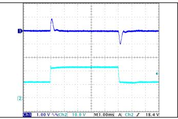
Figure 6: Output voltage response to step-change in input voltage (nominal to maximum), at full load current. Load cap:  $100 \mu$ F, electrolytic output capacitance. Ch 1: Vout, Ch 2: Vin.
