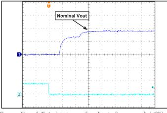
Common Figure 1: Typical startup waveform. Input voltage pre-applied, ON/ OFF Pin on Ch 2. Output voltage normalized.
